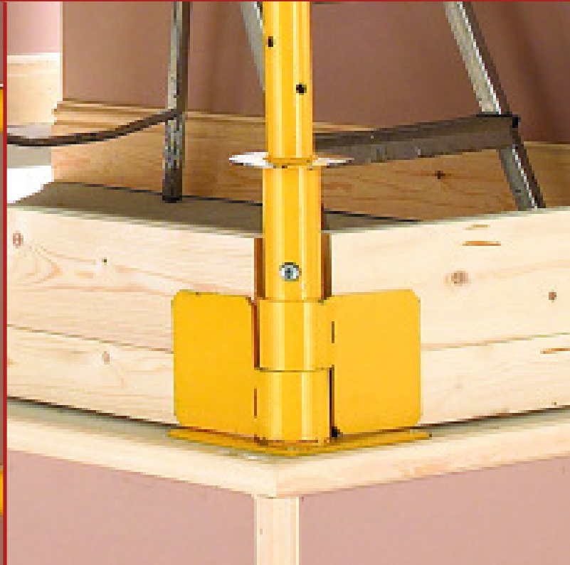
Newel bases are simply screwed into the platform* before slotting over kick board sleeves & installing newels
